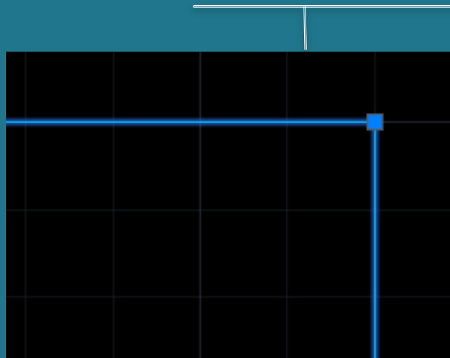
Lines of the same type merged together to become a single polyline
